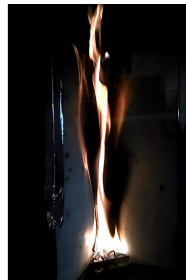
Mini-SBI corner test on HFFR compound based on EVA+ATH+n-MDH or EVA+ATH+antidripping synergist
