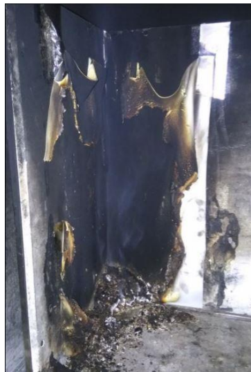
Mini-SBI corner test on HFFR compound based only on EVA+ATH
